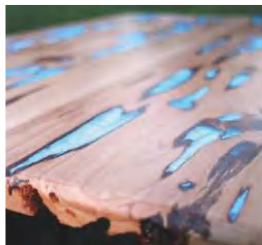
Mike Warren will be showing you how to fill voids with photoluminescent powder in a future issue
